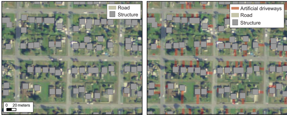
Fig. 2. Comparison of (a) original road network and (b) added segments ("artificial driveways") to connect residential and business population counts to road networks.
